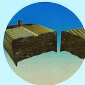
Heat exchanger failure due to limescale. (inset) shows layers of the heat exchanger
