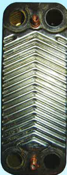
Heat exchanger failure due to limescale. (inset) shows layers of the heat exchanger
